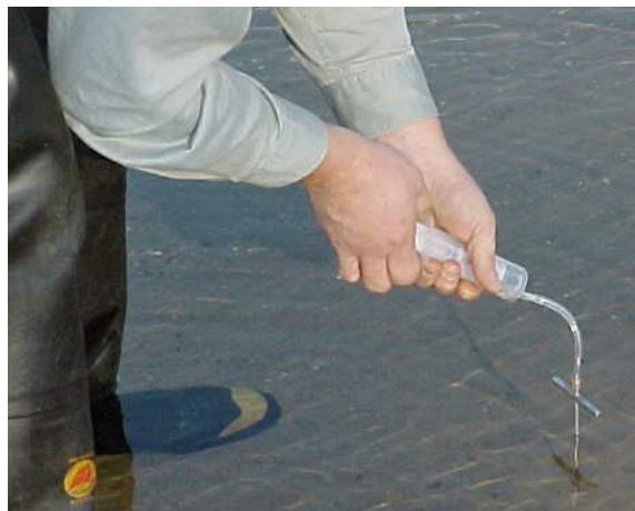
Figure 1: Groundwater Extraction via Pore Water Sampler and Syringe Source: www.mheproducts.com
